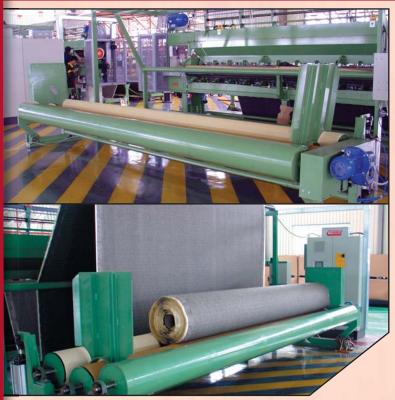
For use at the end of finishing lines and the back of tufting machines. Capable of rolling lengths of carpet in excess of 300 metres.
